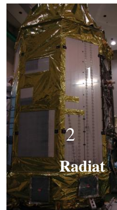
1.HXD-S heat pipe, 2. XIS-S heat pipe
