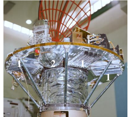
1. Thermal louver, 2. RCS tank.
