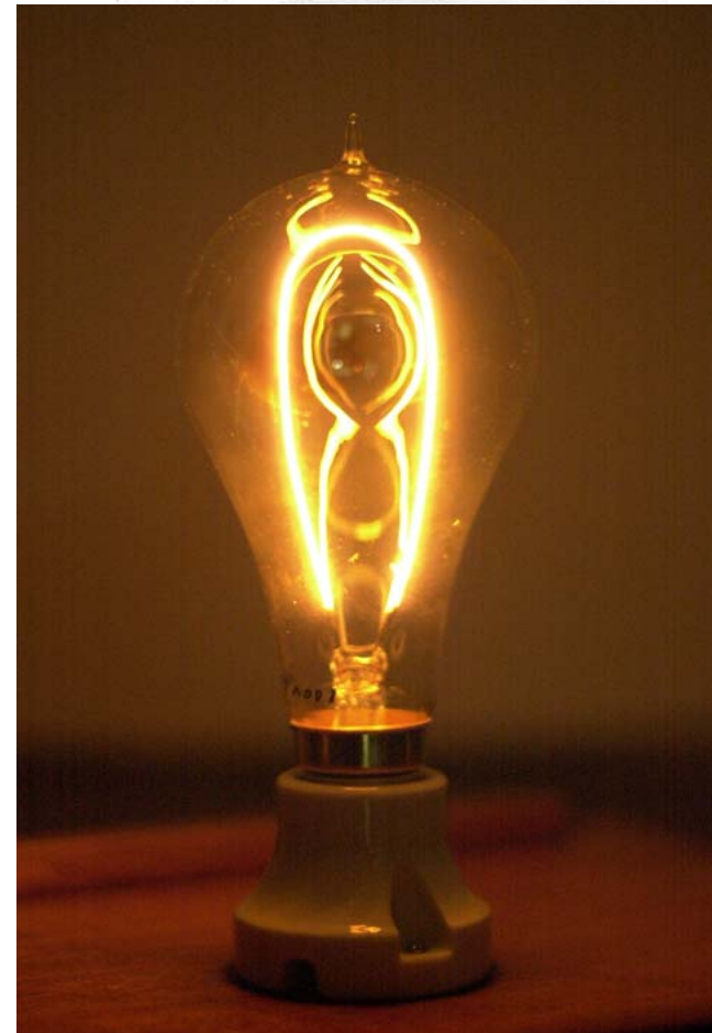
Edison lamp replica Carbon filament made from real bamboo in Yawata city, Kyoto
