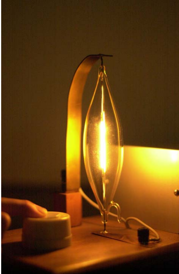
Swan lamp replica Linear carbon filament made from cotton
